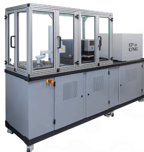
Figure 1. SolidSample ICPMS configured for high-throughput analysis of plastic samples.
